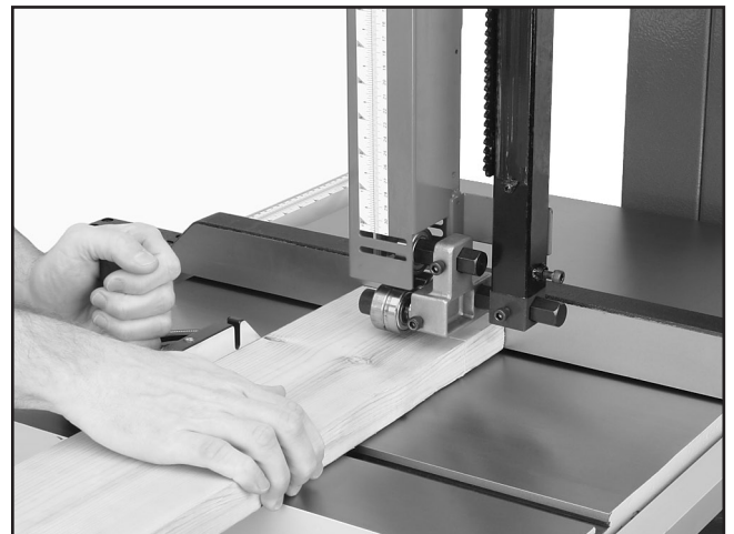
Figure 33. Typical crosscutting operation.
